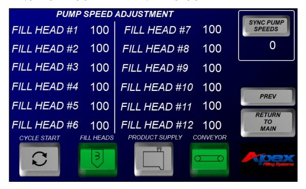
Here you can adjust the pump run speed from 0-100 percent for each head individually that you have enabled.
