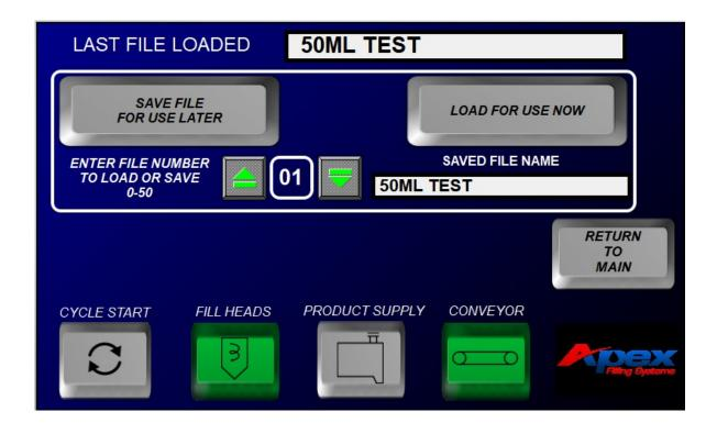
Pressing directly on the numeral will pop up the numeric entry window, or you can press the up or down arrows. Select the desired number (0-50) and either save or load the data by pressing the associated button.
