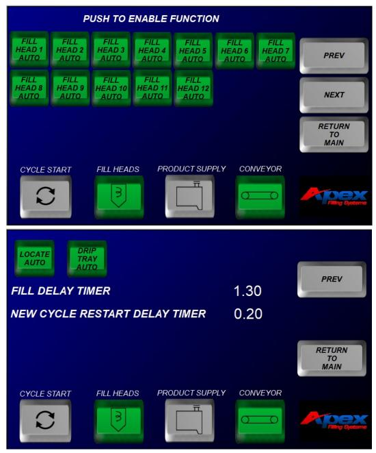
The first fill cycle set-up screen allows the operator to enable or disable fill heads based on machine capabilities. The fill head toggle buttons will switch between OFF and AUTO. The second fill cycle setup screen will allow for further function and timers to be changed. Pressing on any timer description will bring up a pop up with further information.
