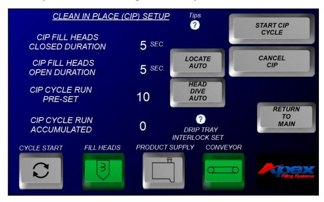
The Clean In Place Screen displays the various programmable parameters for the CIP system and displays the number of CIP cycles completed (when using the CIP Cycle Run)
