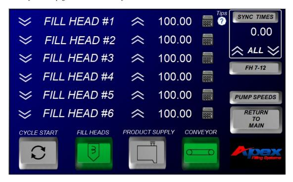
The Fill Head ADJUST screen allows for incremental adjustments to the individual fill head timers up or down by pressing the up or down arrows to the left and right of the associated fill head. The appropriate number of fill heads will be displayed for the machine configuration. If equipped, there will be a screen jumps displayed to access additional fill head timers.
