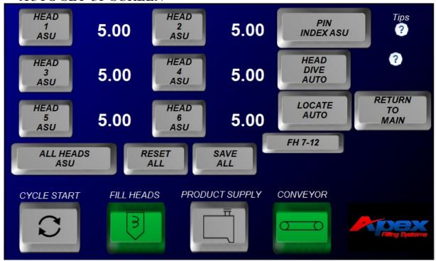
The Automatic Set-Up Screen allows the operator to program fill head times directly by pressing and holding the buttons for the associated fill heads, or pressing ALL HEADS ASU to open all heads and begin the fill process.
