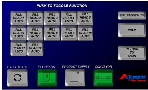
The second manual toggle screen allows the operator to toggle fill heads from automatic mode to manually run.
