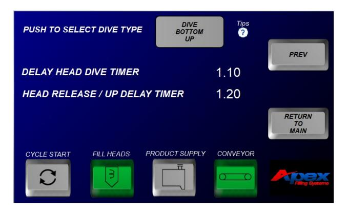
HEAD DIVE TYPE (OFF, STD or DIVE BOTTOM UP) Selects between disabled (stationary) diving heads, automatic/standard operation, or "Bottom Up" fill
