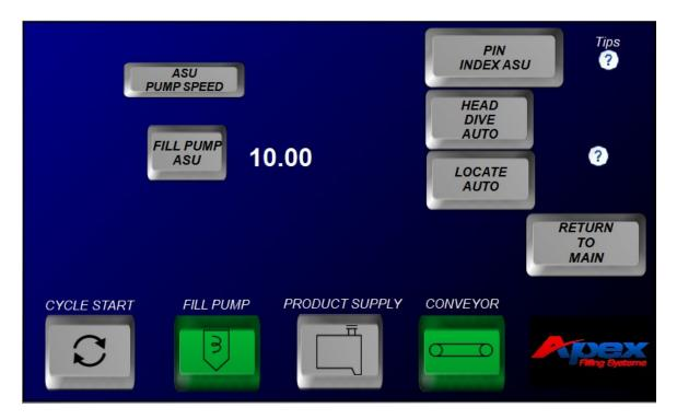
The Automatic Set-Up Screen allows the operator to program fill pump duration time directly by pressing the fill pump asu button and then pressing and holding the fill pump button until the container is filled and overflowing. It is recommended to set the asu pump speed to the highest pump speed you wish to run during an auto cycle. Running the asu will give you a baseline number to then fine tune during an auto cycle. This does not account for any ramp settings.
