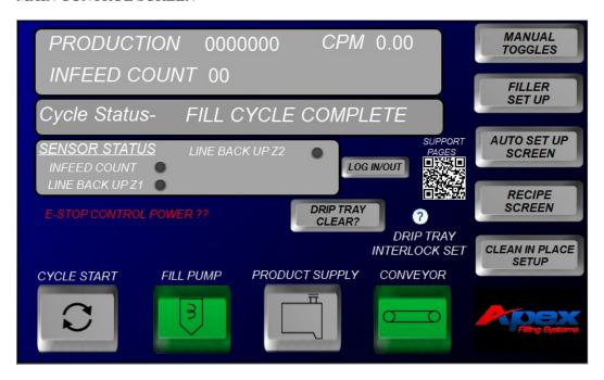
The main screen of the controller provides the primary filler function status at a glance.
