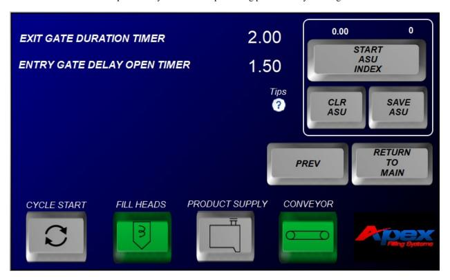
Basic sequence of ASU indexing setup (pin indexing):
