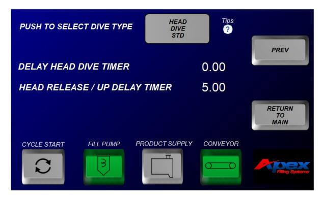
HEAD DIVE TYPE (OFF or STD) Selects between disabled (stationary) diving heads or automatic/standard operation
