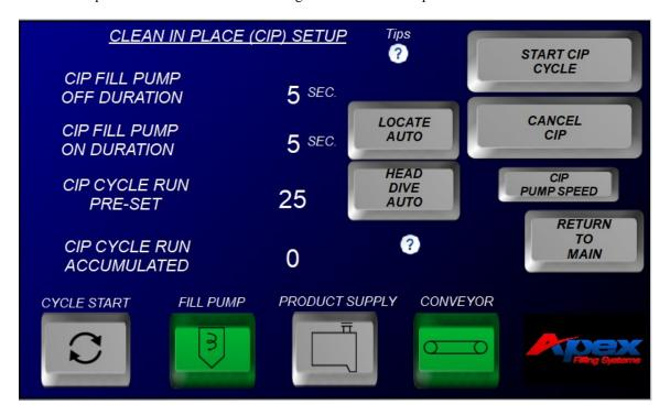
The Clean In Place Screen displays the various programmable parameters for the CIP system and displays the number of CIP cycles completed (when using the CIP Cycle Run)
