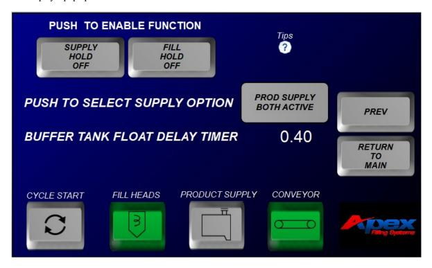
FILL HOLD (OFF or ON) Enables or disables the fill hold option. If enabled, filler will wait until float is satisfied before next cycle
