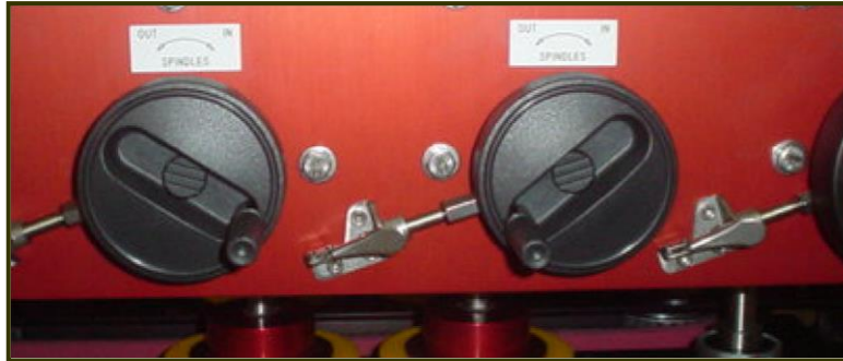
Figure 12. SPINDLE WIDTH ADJUSTMENT CONTROLS.
