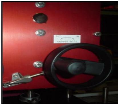
Figure 17. GRIPPER BELT WIDTH CONTROL.
