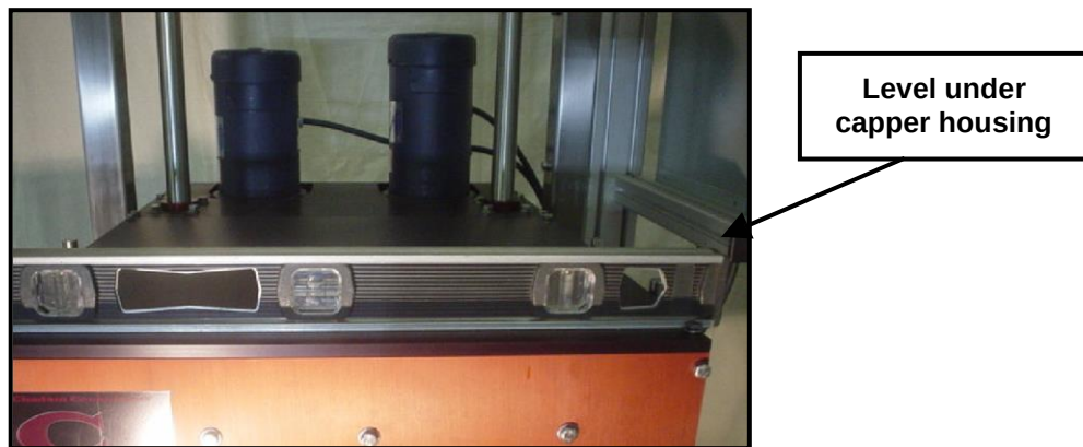
Figure 8. LEVEL THE CAPPER HOUSING FROM SIDE TO SIDE.
