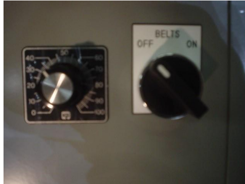
Figure 6. GRIPPER BELT POWER AND SPEED CONTROLS.
