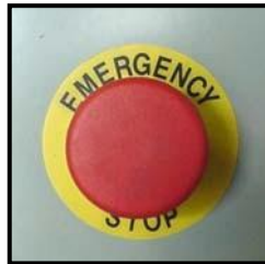
Figure 2. EMERGENCY STOP (E-STOP) BUTTON.
