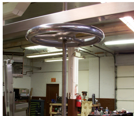
Figure 4-7 Fill Bar Height Adjustment
