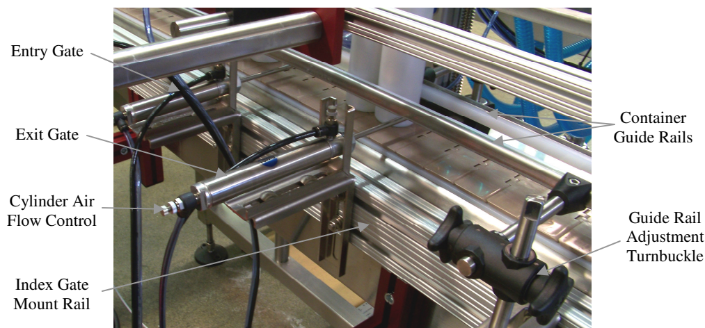
Figure 4-3 Guide Rails and Indexing Gates
