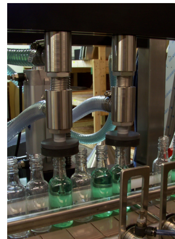
Figure 4-11 Nozzle Fully Compressed
