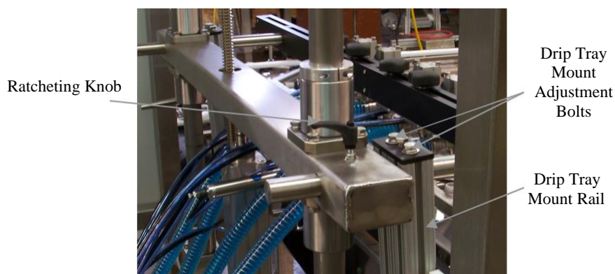
Figure 4-6 Fill Bar and Drip Tray In/Out Adjustment
