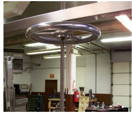
Figure 4-7 Fill Bar Height Adjustment
