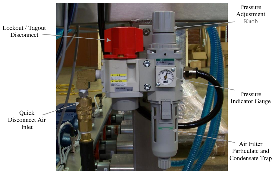
Figure 3-3 Main Air Disconnect and Filter Regulator
