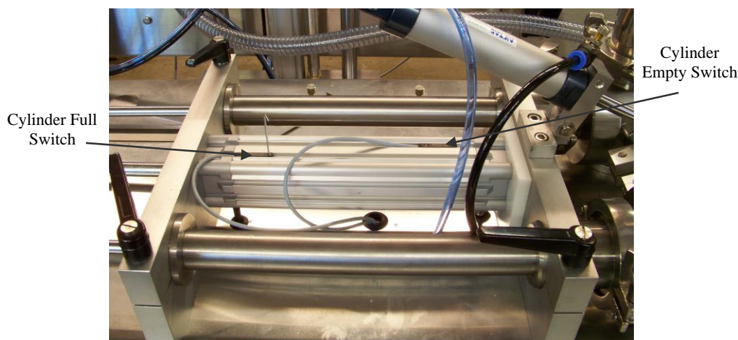
Figure 5-8 Magnetic Reed Switches (Cylinder Position Sensors)
