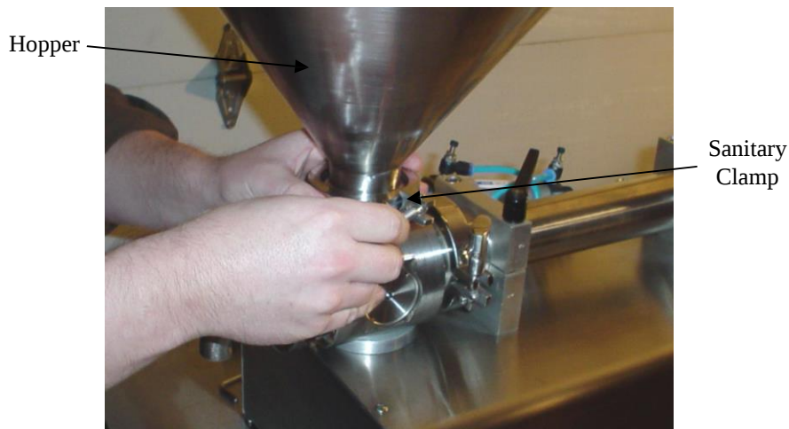
Figure 5-1 Hopper Tank Removal
