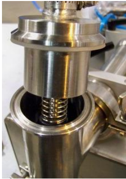
Figure 5-12 Fill Check Valve
