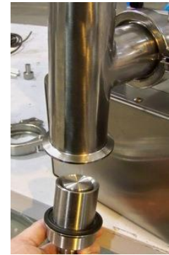
Figure 5-13 Inlet Check Valve
