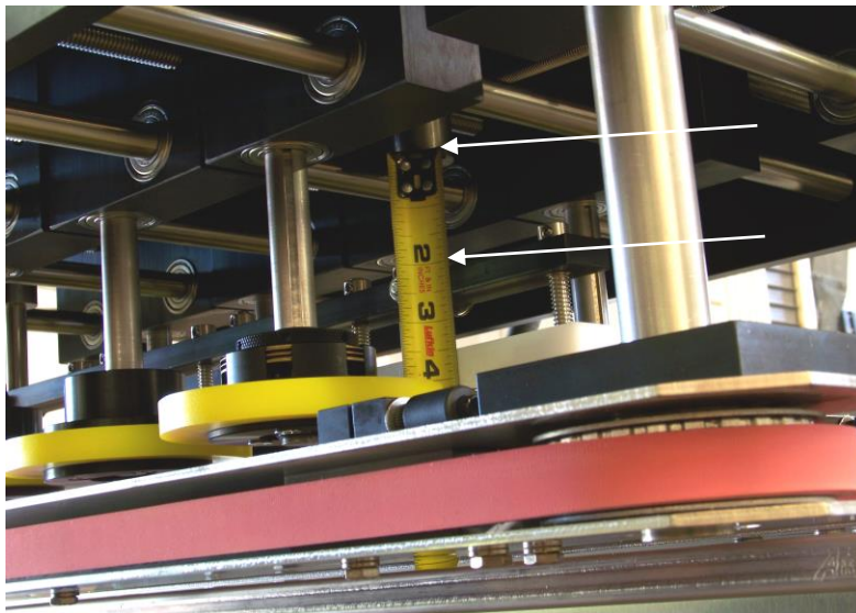
Figure 8-5 Cap Stabilizer Height
