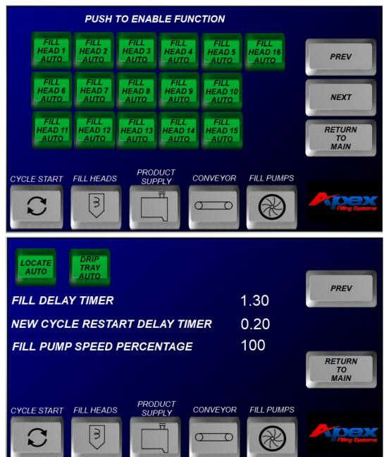
The first fill cycle set-up screen allows the operator to enable or disable fill heads 1 thru 16. The fill head toggle buttons will switch between OFF and AUTO. The second fill cycle setup screen will allow for further function and timers to be changed. Pressing on any timer description will bring up a pop up with further information.
