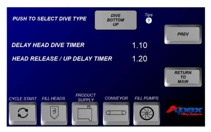
HEAD DIVE TYPE (OFF, STD or DIVE BOTTOM UP) Selects between disabled (stationary) diving heads, automatic/standard operation, or "Bottom Up" fill
