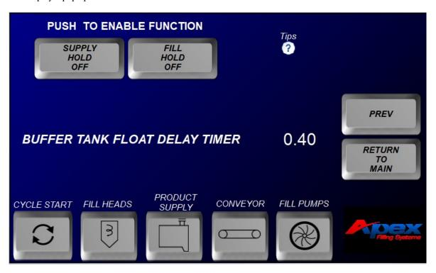
FILL HOLD (OFF or ON) Enables or disables the fill hold option. If enabled, filler will wait until float is satisfied before next cycle
