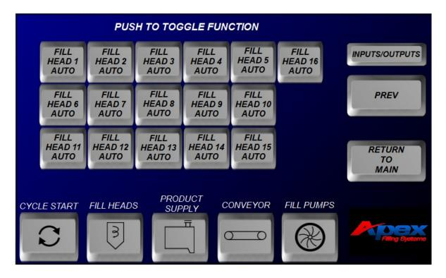
The second manual toggle screen allows the operator to toggle fill heads 1 thru 16 from automatic mode to manually open.
