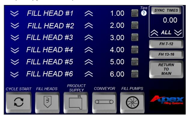
The Fill Head ADJUST screen allows for incremental adjustments to the individual fill head timers up or down by pressing the up or down arrows to the left and right of the associated fill head. The appropriate number of fill heads will be displayed for the machine configuration. If equipped, there will be a screen jumps displayed to access additional fill head timers.
