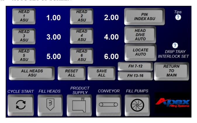
The Automatic Set-Up Screen allows the operator to program fill head times directly by pressing and holding the buttons for the associated fill heads, or pressing ALL HEADS ASU to open all heads and begin the fill process.
